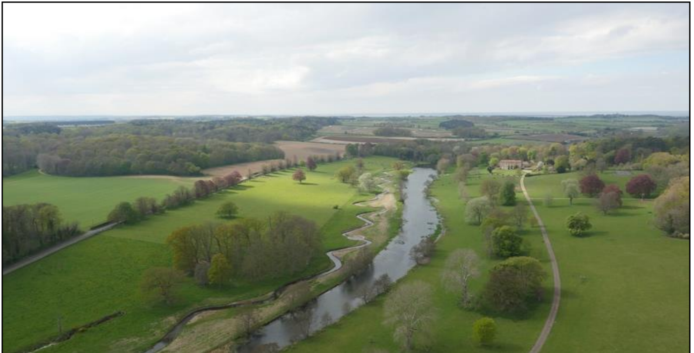
Fig. 1: A new channel created for the River Glaven, winding its way to the left of Bayfield House Lake in Norfolk, the product of a multi-party project managed by the Wild Trout Trust (photo: flypodimagery.com).
