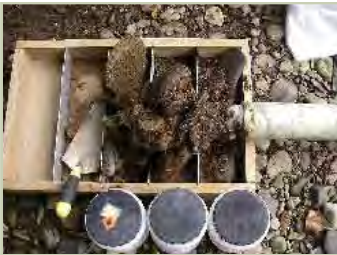
FREEZE CORE SAMPLING TO ASSESS QUALITY OF SPAWNING GRAVEL
