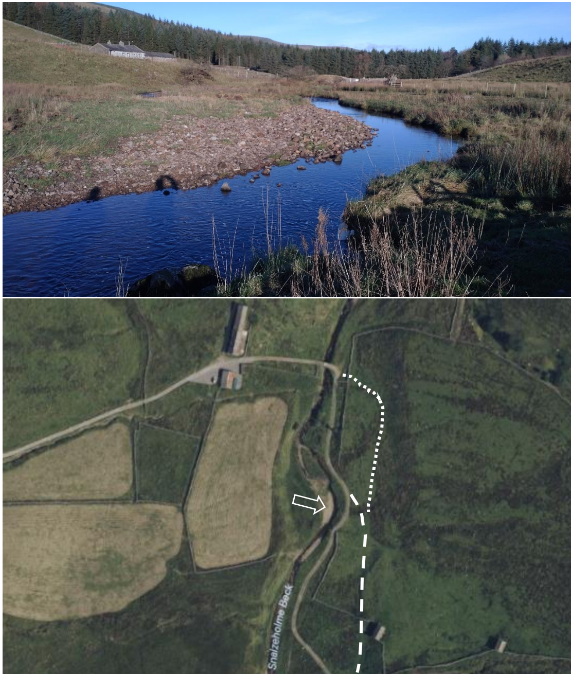
Fig 2. An unconsolidated deposition bar of boulder, cobble and gravel points to the dynamic nature of the channel here, highlighted by the white arrow in the satellite image. Historically, a track was formalised using material from the riverbed, running close and parallel to the channel on the RB and the channel straightened. A new track to the barn has been laid further away (indicated by the dashed line), but it is worth considering whether it could be moved even further (eg on the dotted trajectory from the bridge), allowing for renaturalisation of the riparian zone. NB flow direction: south to north.
