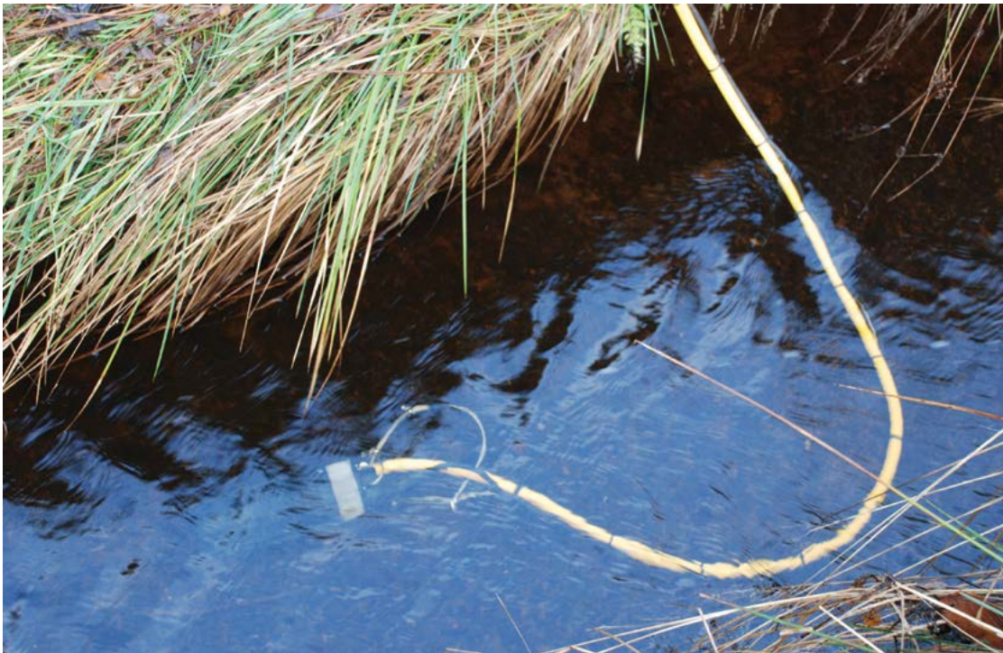
Figure 4.27 A water sampler at Knapdale. Public health monitoring for the SBT involved taking water samples from four to five sites every three months, and testing for Giardia and Cryptosporidium 29 . © Argyll and Bute Council
