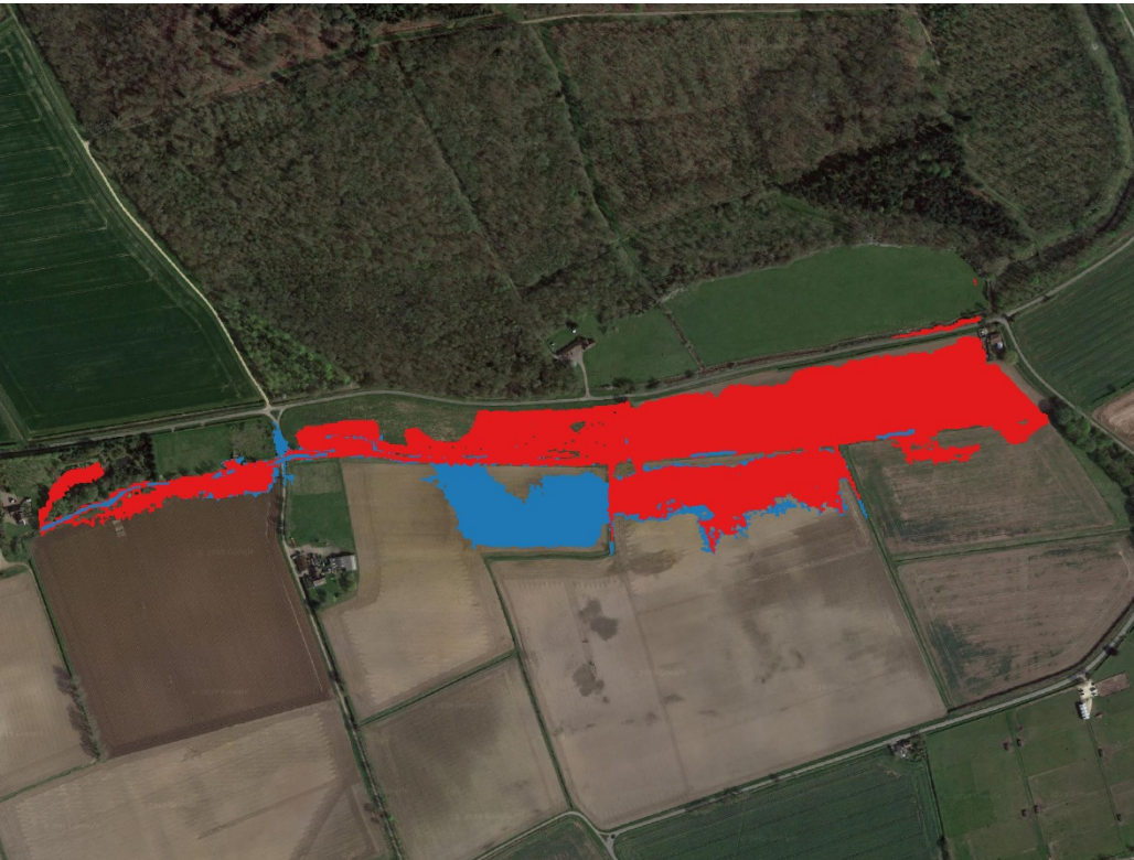
Figure 4.6b 1 in 20yr flood extent change, blue = baseline, red = restored (where blue is visible indicates flood extent decrease).
