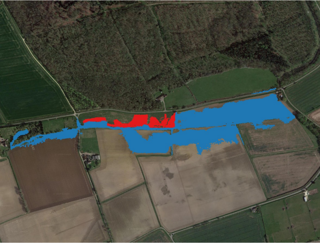
Figure 4.6a 1 in 20yr flood extent change, blue = baseline, red = restored (where red is visible indicates flood extent increase).
