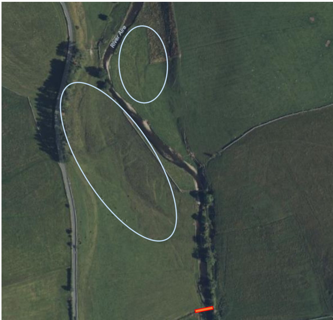
Fig 1. D/s limit of the beat (red bar), the extant Aire channel was shunted in straightened sections through the floodplain and then pinned against the eastern side to provide head at a weir d/s. Note in contrast, the sinuosity of the paleochannels in the floodplain (ringed). The deposition bars of exposed cobble, maintained bare by livestock, were also obvious from this perspective.
