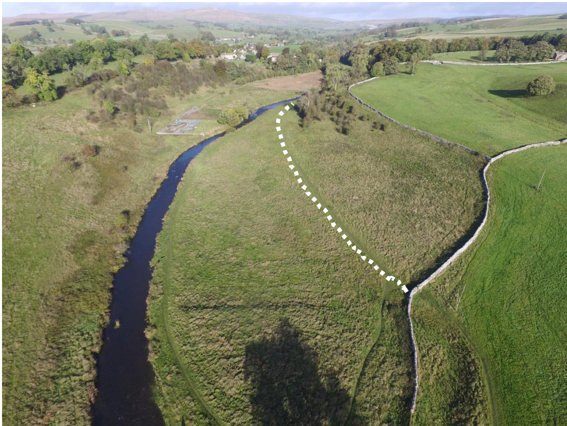
Fig 14. Pre works drone flight over the upper reach highlighting the long sweeping engineered bend and the desire line of footfall running parallel to the bank top. White dotted line indicates the fencing to keep people on the Pennine Way, and the area given over for renaturalisation. 18mo prior to this image, all the grass along the river looked like the closely grazed sward in adjacent fields.
