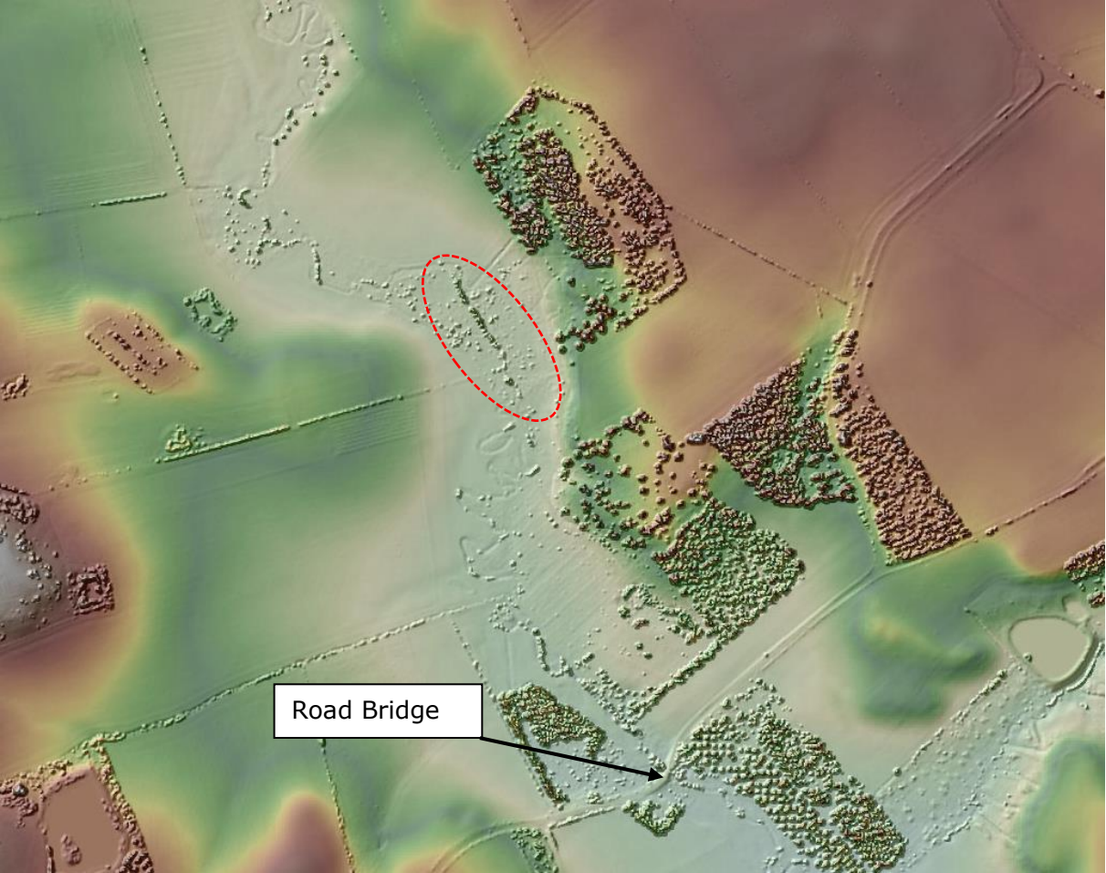
Figure 35 Another section of the Bain (red ellipse) which appears to have been straightened and is possibly a candidate area for restoration.
