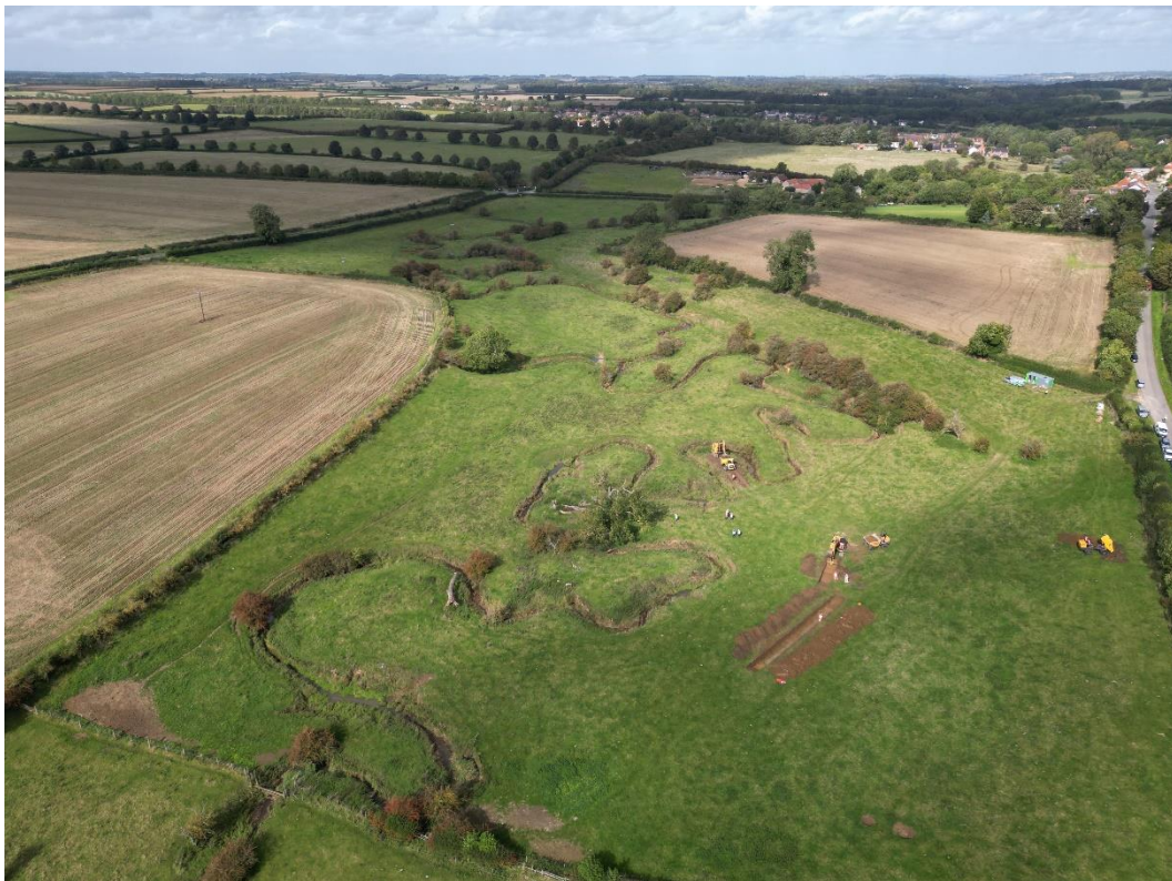
Figure 32 Upper Witham, Colsterworth, pre-project. A sinuous but deeply incised channel disconnected from its floodplain.
