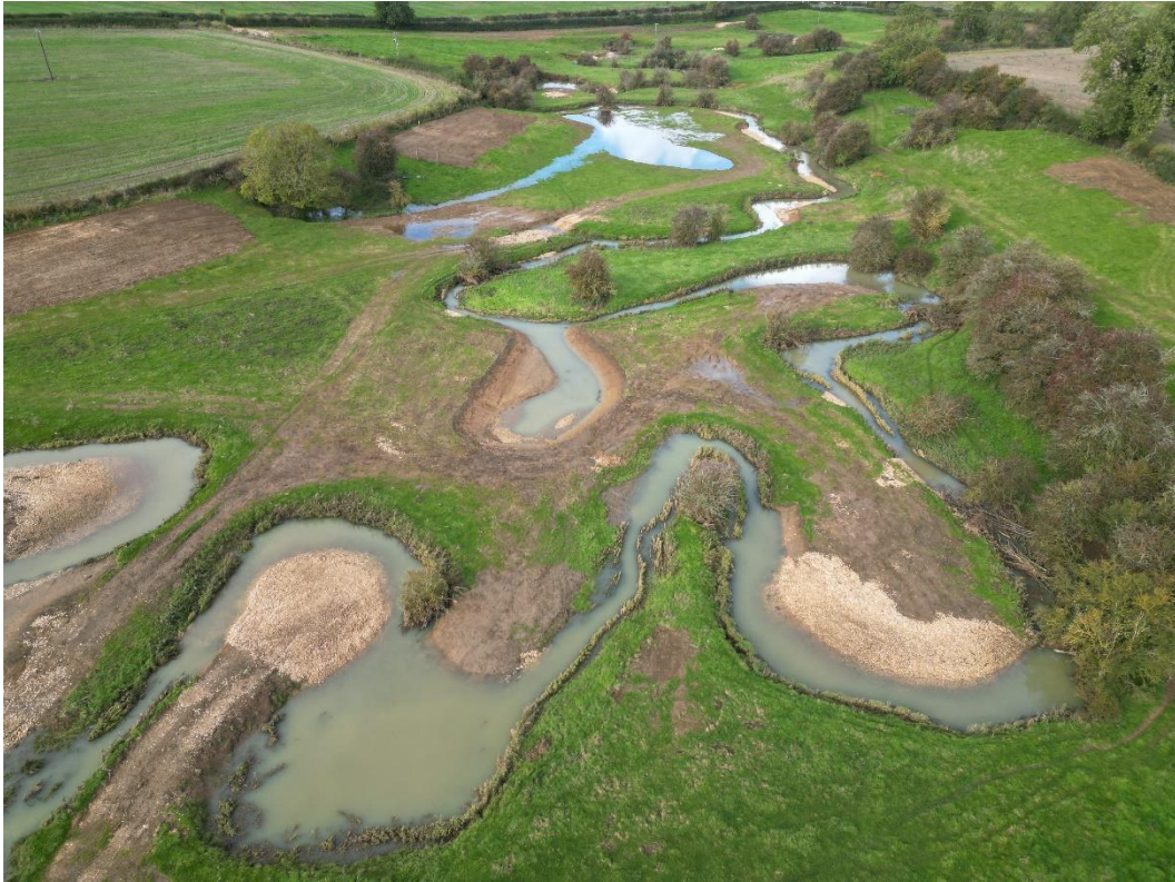
Figure 33 Colsterworth post-project showing bank-reprofiling (inside of meanders), gravel introduction, backwater creation. River flow is away from camera.
