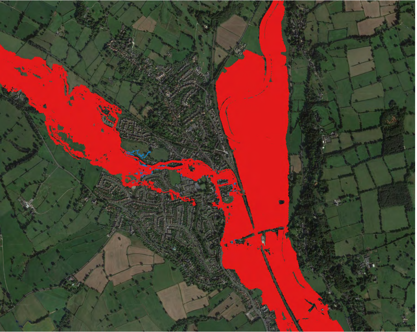
Figure 4.2b 1 in 100yrCC flood extent change, blue = baseline, red = restored (where blue is visible indicates flood extent decrease).
