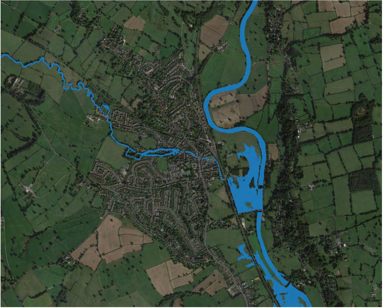
Figure 4.3a 1 in 5yr flood extent change, blue = baseline, red = restored (where red is visible indicates flood extent increase).
