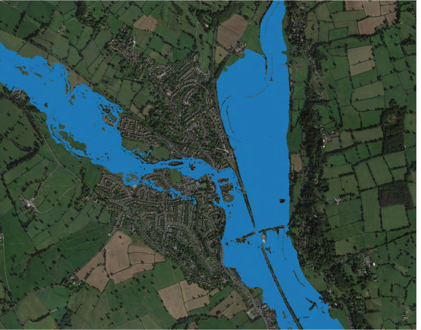
Figure 4.2a 1 in 100yrCC flood extent change, blue = baseline, red = restored (where red is visible indicates flood extent increase).
