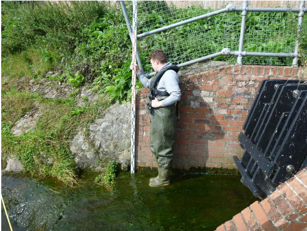
Photo 2 Temporary benchmark position, NGR SK4528247570, nominal level 3.3m
